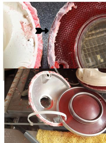
Keep each lens and housing together. You may wish to use a plastic tie or string to keep them together. This ensure the lens and housing
