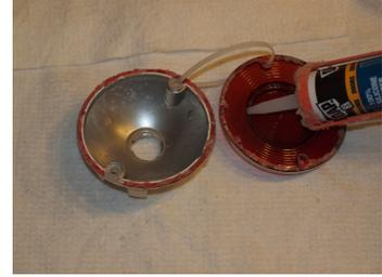
The lens and housing will be squeezed together when you install them. This will keep the lens and housing from separating. The silicon is to keep the system somewhat water tight.
