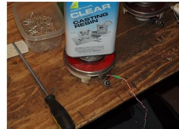
As with the reverse lens, place a bead of silicon around the housing's edge, align the mark and press the lens and housing together. Use a weight to ensure the silicon is allowed to dry without the lens moving.
